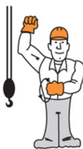
Crawler Crane Travel One Track
