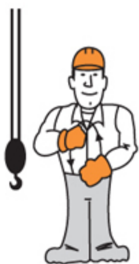
Crawler Crane Travel Both Tracks
